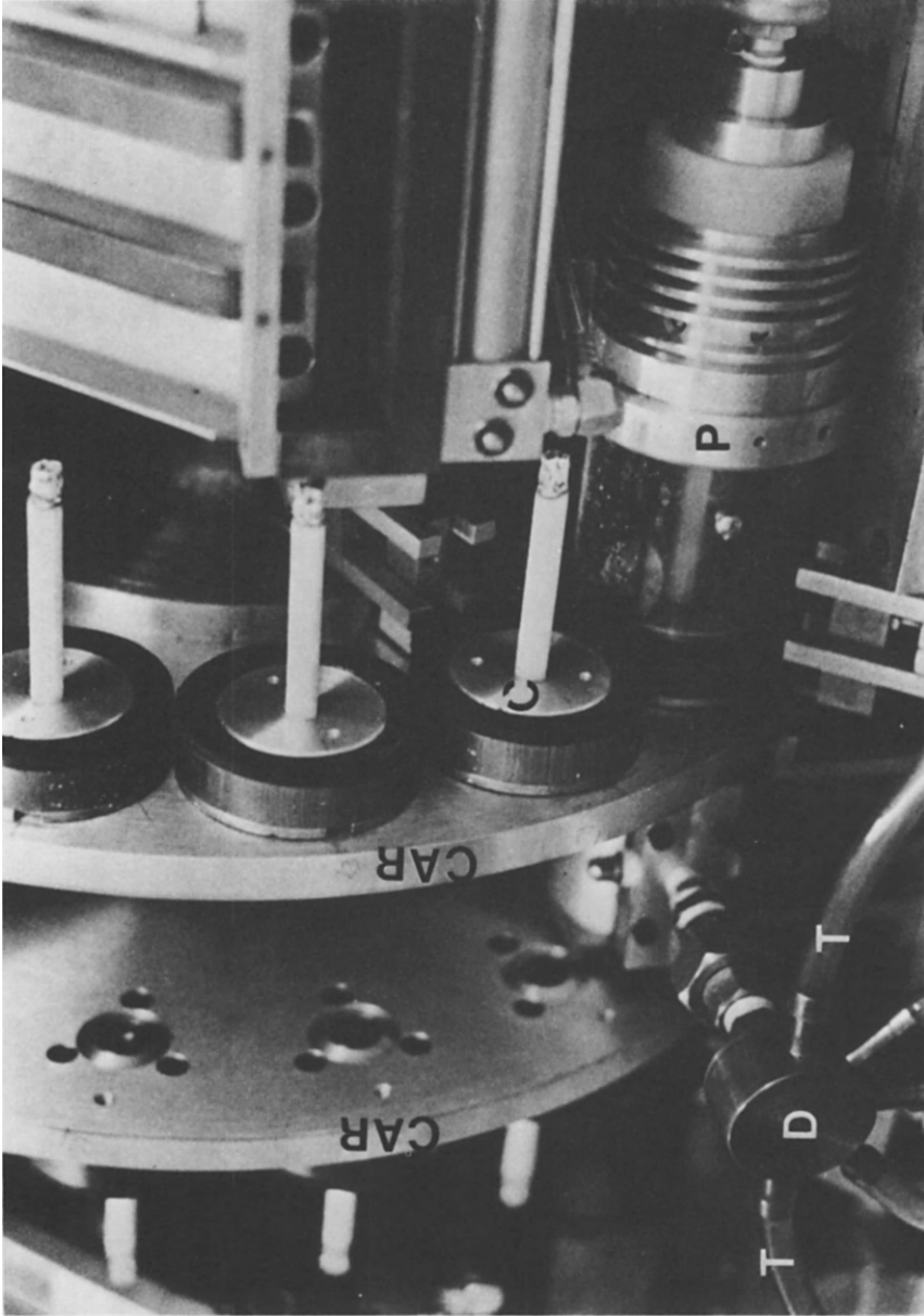
FIG. 2. Detail of smoke-generating machine. The puff chamber (P) delivers a 35 ml standard puff volume. Cigarettes are held by collets (C) arranged on a pair of rotating carousels (arrows). The freshly generated smoke is diluted 1 : 10 with a supply of carbon monoxide-free air (A) and partitioned to the channels of the animal exposure rack by the distribution valve (D). The smoke-generating machine is connected to the exposure rack by polyurethane tubing (T).
