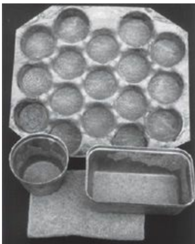
BOARDS AND CONTAINERS FROM HEMP HURDS. PHOTOGRAPH COURTESY OF INSTITUT FÜR ANGEWANDTE FORSCHUNG.
