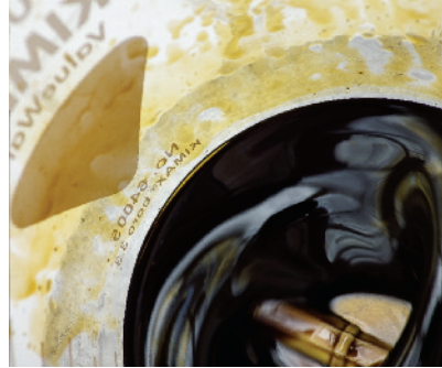
21. You can control the speed of the magnetic stirrer bar. Keeping your oil moving helps to avoid 'hotspots.'
