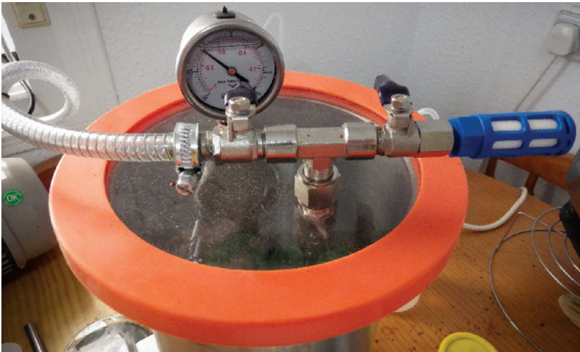
22. By using a vacuum chamber you can remove all the traces of butane to create 'shatter.'
