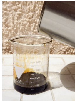
17. Switch off before all the solvent and (after leaving to cool) carefully pour into a suitable receptacle.
