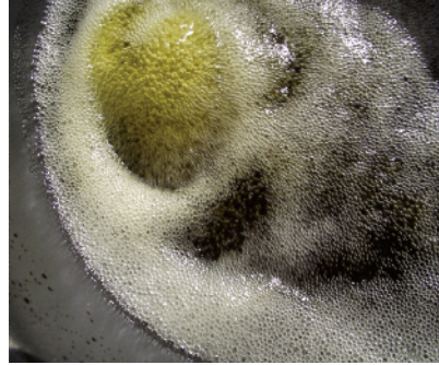
15. The boiling solvent will be very volatile and there is a risk of explosion. So, no naked flames!
