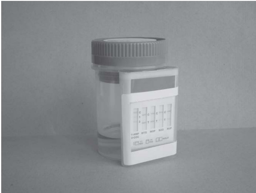
Figure 6.2: Sealable specimen cup with built-in testing strips
