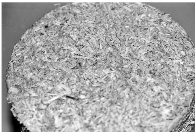
Fig. 17.6. Test tube of hemp cement – surface view.
