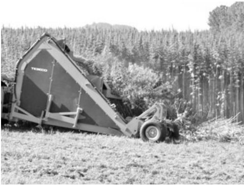
Figs 6.5 and 6.6. Mowers cutting at two and three levels with a working width of 4 m. These are manufactured by Tebeco (Tebeco ©, 2009).
