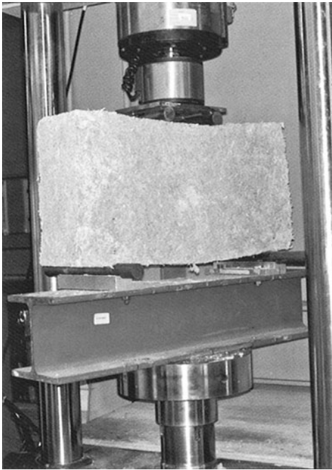
Fig. 17.9. Flexion tests on hemp bricks.
