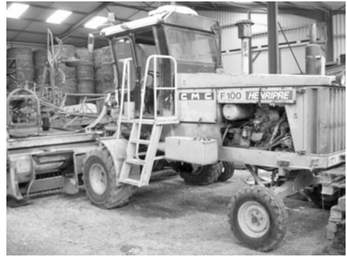
Fig. 6.7. Automatic 'swather cutter', initially used for harvesting lucerne (ITC ©).
