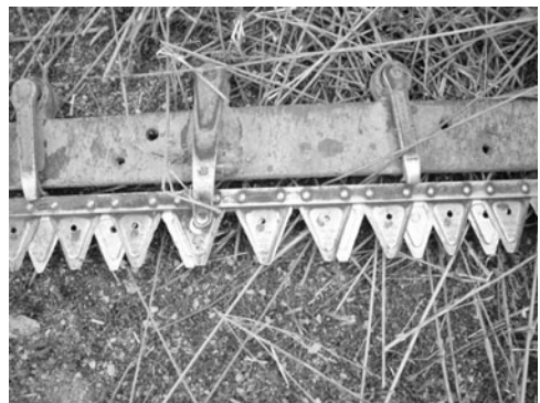
Fig. 6.4. Double knife-cutting system (Busatis, ITC®).
