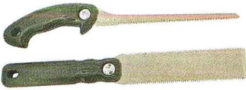
Two saws: one (flat) for cutting boards and one for cutting holes. You can also use a power saw.
