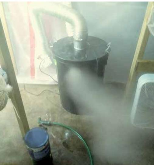
▲ A DIY pond fogger—a 10-head ultrasonic hydroponic fogger on a float in a trash can. Fan-forced air ducted in the top pushes mist out a hole in the side. DALLAS LAWLOR
