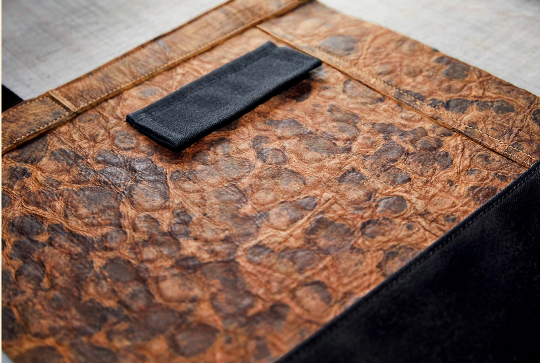
Mylo™, a leather-like material made from mycelium cells, created by Bolt Threads.
