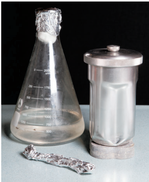
Liquid agar can be sterilized in an Erlenmeyer flask (stuffed with Poly-fil and covered with foil), along with foil-wrapped tweezers and blender parts.
