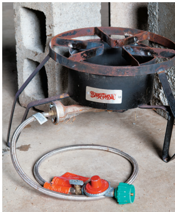
A large propane-fired burner is used to pasteurize the straw. Place the barrel on cinder blocks surrounding the burner for better support.
