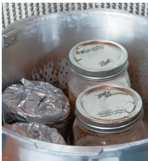
Agar can also be sterilized in mason jars (along with stacks of glass petri dishes wrapped in foil).
