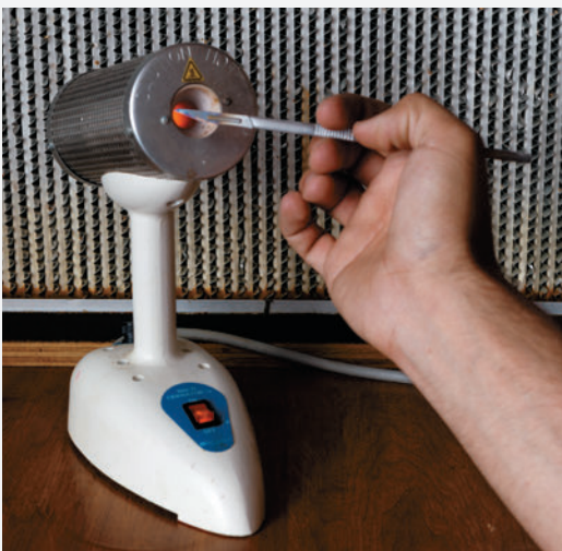
Scalpels can be sterilized in a pressure cooker or with an infrared sterilizer such as the one shown here.
