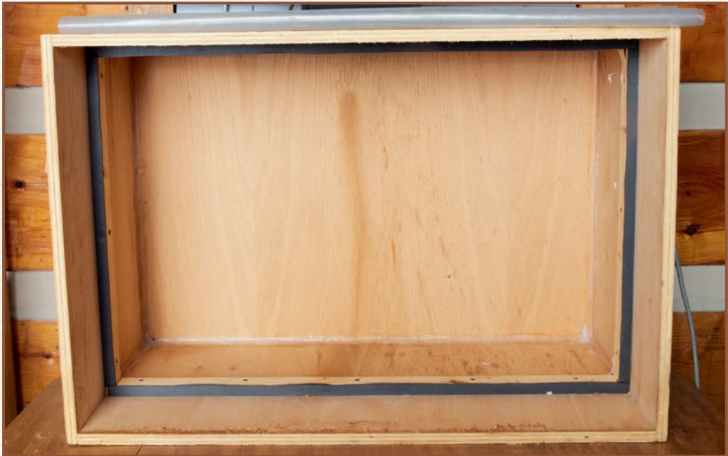
The finished flow hood box is ready for the filter to be installed.
