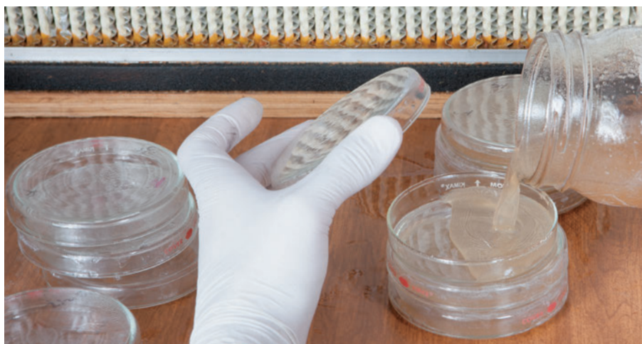
Once both the agar and the petri dishes have been sterilized, pour just enough of the agar to cover the bottom of the dish with about an \frac{1}{8} -inch (0.6 cm) layer.
