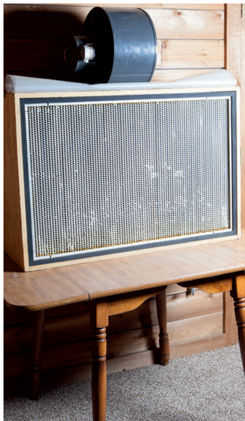
A flow hood with a HEPA filter creates a flow of sterile air, which will allow you to perform sterile procedures directly in front of it.
