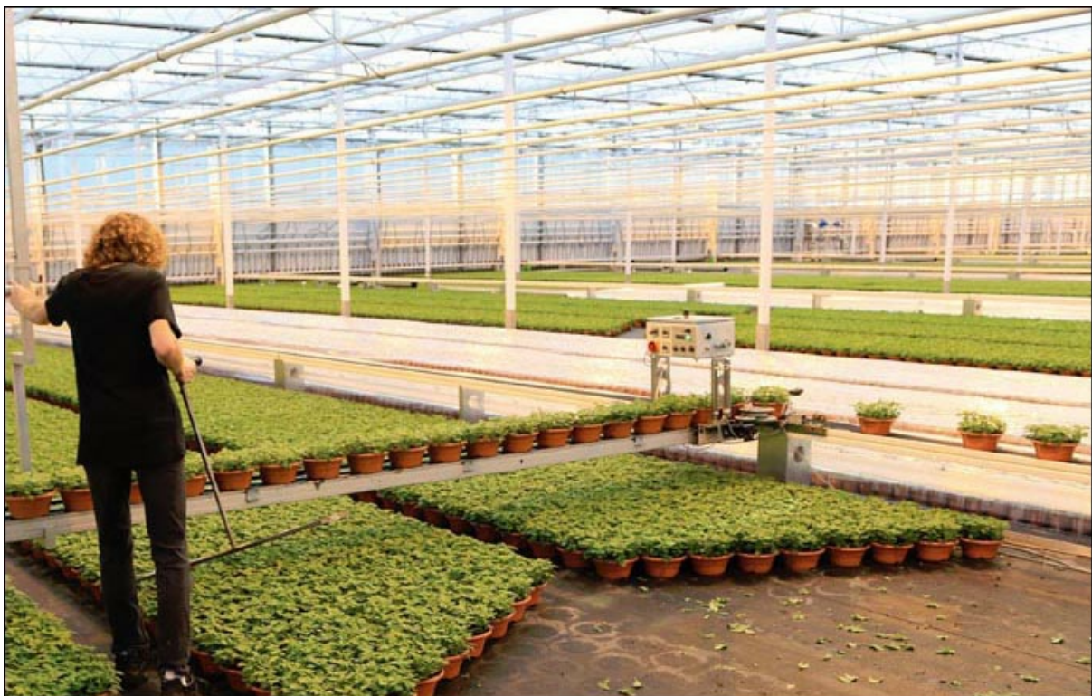
The SmartFlo system of WPS, The Netherlands, consists of several modules of conveyors that are connected online. The SmartFlo Flexit, one of the essential elements of SmartFlo, is a flexible conveyor belt that is easy to install and relocate. [2017]
