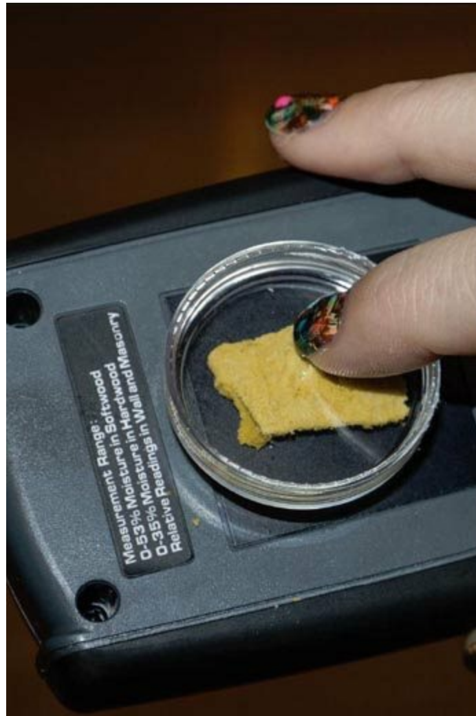
A piece of compressed kief. We used plastic, glass and metal plates to separate finger from the material. The readings seemed to be more accurate.
