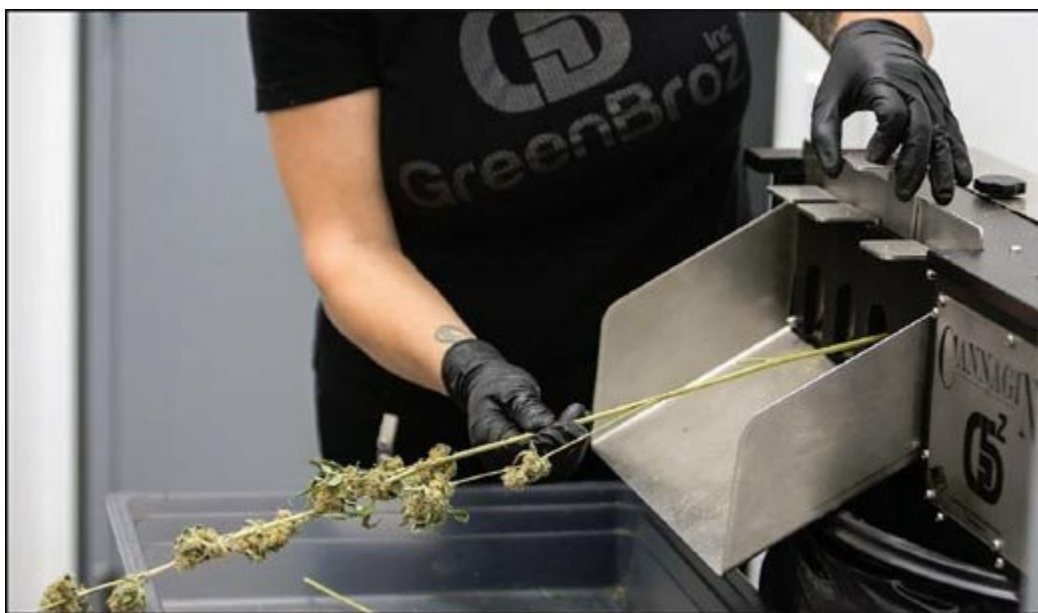
Bucking Machine by Greenbroz makes short work of removing buds from stems. The operator
