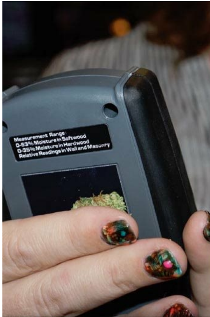
A photo of the first trial of the moisture meter. We found that the moisture in the finger can affect the reading. (Photo model: Ellen Holland)
