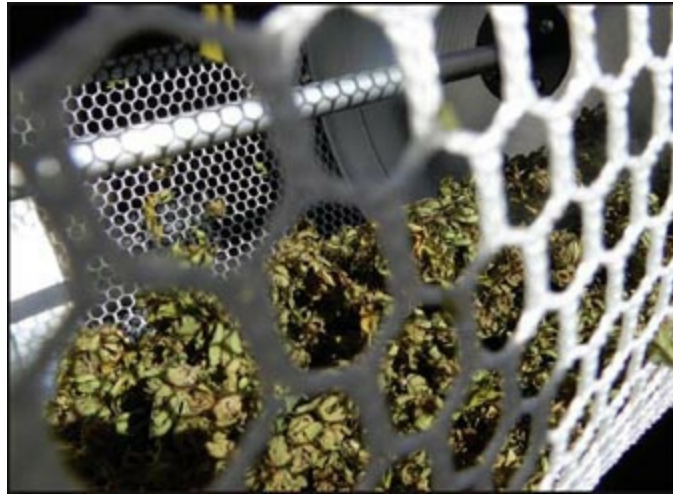
Close-up of Tom's Tumbler showing net that forms a drum.
