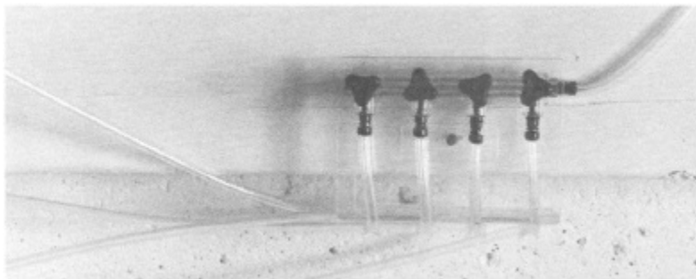
Plate 7. Multiple air valve. Make sure that it has the same number of air valves as growth tanks in the system.
