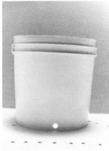
Plate 9. \frac{3}{8} " hole as close to the bottom of the growth tanks as possible.
