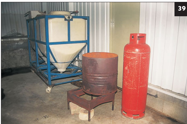
39 Equipment used for formalin fumigation. The large metal container holds the formalin and a bottle gas supply provides the fuel for the heat for vaporization.
