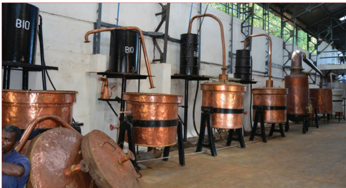
Stills used to produce ylang-ylang essential oil in Nosy Be, Madagascar
