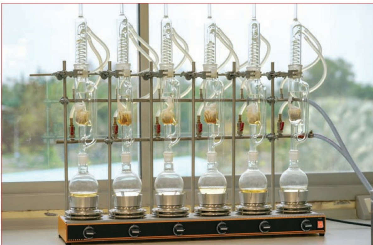
Soxhlet extractor used for extraction by solvents
