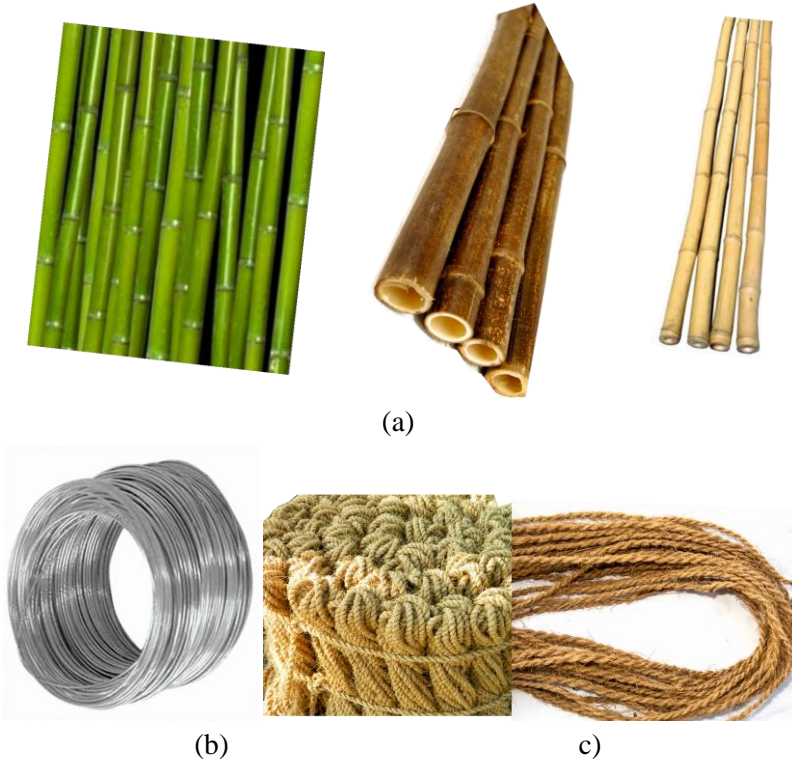
Figure 56. Bamboo pole (a), iron wire (b) and coconut thread (c) commonly used in betel vine garden (or Boroj) construction.
