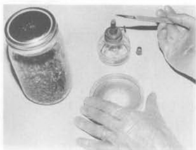
fig. 33: Flaming the scalpel.
