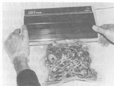
fig. 53: Bags are heat-sealed with a bag sealer.
